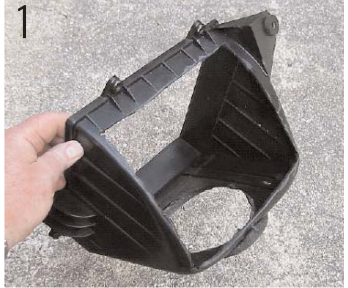
1 Lower half of the airbox. The section to cutout is the solid piece facing the front of the car.
