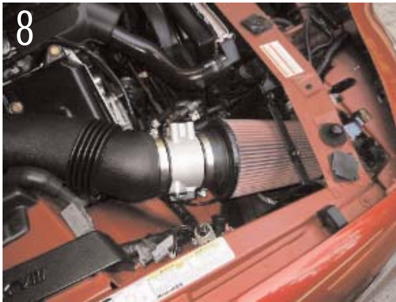
Now install the new MAF and filter. Be sure the MAF is rotated about 45% as shown.
