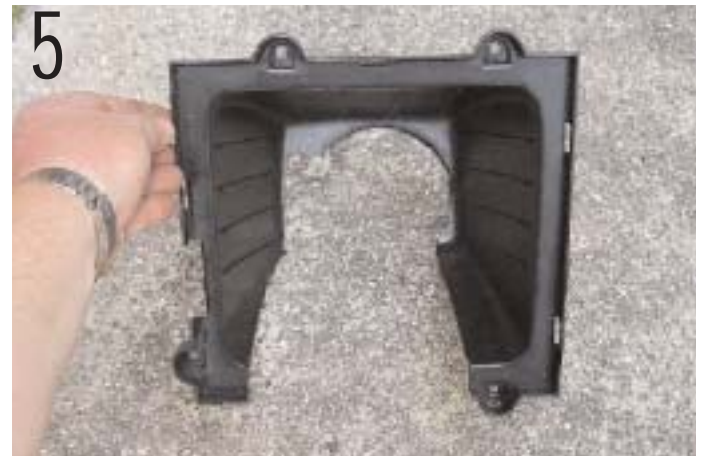
5 A view of the airbox top looking from the car's nose back. The top of the box is the top of the picture
