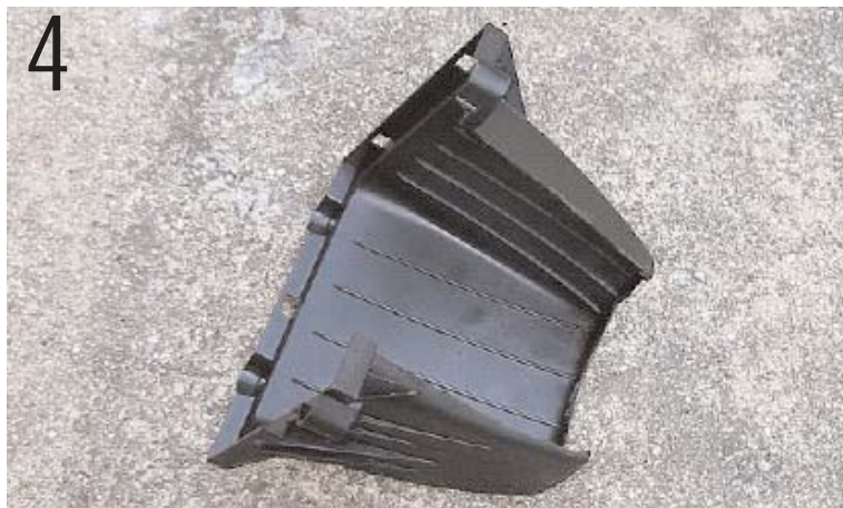
4 This is the bottom of the top half of the airbox. You need to completely cut this piece out.
