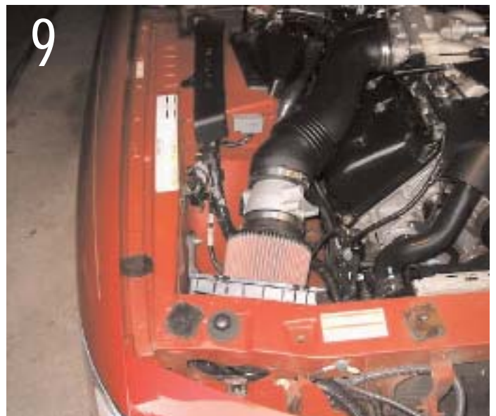
Another view of the MAF and filter installed.
