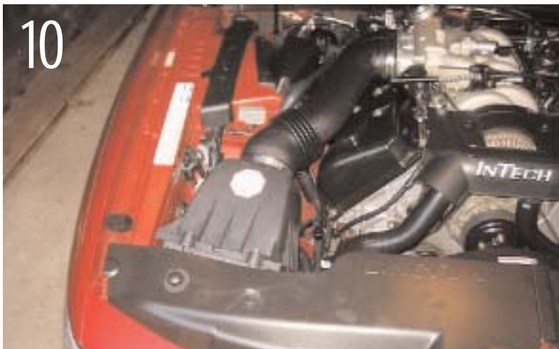
Now position the top half of the airbox over the MAF and use the top bolts to attach it to the bottom half. The new MAF and filter float inside.
