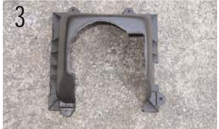
3 This is a view of the cutout needed for the rear facing section of the top half of the airbox. The top of the piece is at the top of the picture. The section to cut is the part that has the collar that attaches to the air tube leading to the throttle valve.
