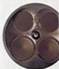
Each cylinder's combustion chamber breathes in and out freely through four valves.
