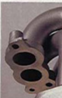
Dual tuned runners deliver air to each cylinder to optimize both low- and high-speed performance.
