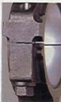
Connecting rod bearing caps are mechanically fractured so they can be reassembled only one way, precisely.
